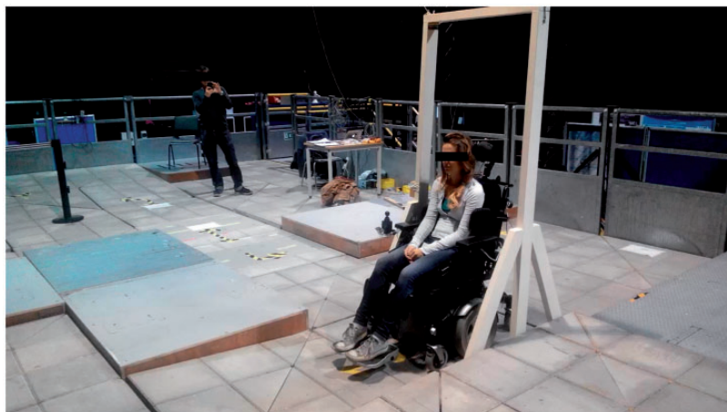
Figure 12. Assessment course used to compare control interfaces (joystick, head-array and sip/puff switch) by evaluating user's driving performance when using the interfaces to complete various tasks. The tasks are similar to those a regular wheelchair user may perform in his/her daily life.
